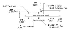
Vertical Orientation PCB Layout (Ref.) from Component Side
