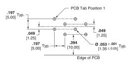
Right-Angle Orientation PCB Layout (Ref.) from Component Side
