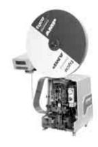
Semiautomatic bench crimping machines that also strip the wire, and are therefore used for terminating jacketed cable. Feature manual precision adjustment of crimp height, keyed strip blades for faster, more accurate setups, and an efficient scrap removal system. All adjustments can be made from the front of the machines without special tools. Available with crimp quality monitoring.
