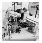
Fully-automatic machines that measure, cut, strip and terminate single leads. Microprocessor-controlled, and programmed and operated using an easy-to-follow, menu-driven touch-screen. Features include directdrive terminating units with precision crimp height adjustment, fully programmable setups, wire runout and splice detection, and motorized pre-feed with wire straightener. Crimp quality monitoring is also available. For more information, request Catalog 124324.
