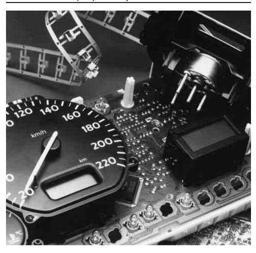
The Printed Circuit Board Pin Receptacle provides a reliable and cost effective means of attaching components with pin contacts to a printed circuit board. Components are held in place without solder allowing for their easy removal from the printed circuit board for replacement or repair. Receptacle contacts are inserted and securely clinched to the printed circuit board by means of semiautomatic or automatic machines.
