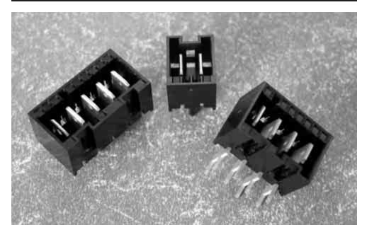
The FASTON RAST 5 Tab Header Assembly system is designed to provide a RAST 5 interface to a Printed Circuit Board. The RAST 5 Standard defines and standardizes the connector mating interface. 250 Series Tabs are placed on 5mm center lines with a plastic shroud that has keying, polarization, and locking features that help prevent mismating of the corresponding RAST 5 female receptacle housing. The header assembly is
