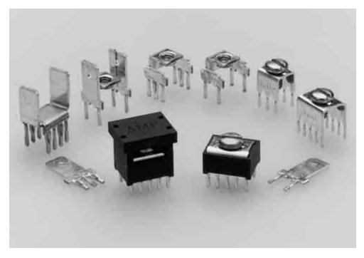
Tyco Electronics Power Taps are designed for the growing need for power to printed circuit board applications required in today's electronic industry. The taps provide a high current, separable connection to a pc board. Pin configuration is of the standard DIP outline with .300 x .100 [7.62 x 2.54] or .250 x .125 [6.35 x 3.18] for the Standard versions, plus .400 x .200 [10.16 x 5.08], .300 x .100 [7.62 x 2.54] and in-line spacing for the High Current versions.
