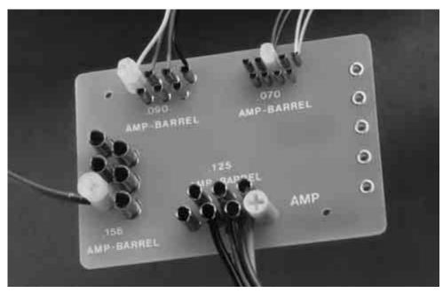
**AMP-BARREL Terminals** solve the problem of interconnecting discrete wires to printed circuit boards without permanently soldering them in place. and provide cost savings by eliminating the need for two-piece terminal systems, terminal strips or expensive space-consuming modular connectors.
