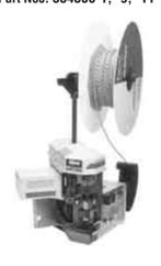
Semiautomatic bench machines for crimping reeled terminals and contacts, featuring a quiet and reliable direct motor drive. microprocessor controls for ease of setup and operation, and guarding and lighting designed for operator convenience. All models are equipped with either manual or automatic precision adjustment of crimp height. Machine-mounted sensors are available for crimp quality monitoring using conventional miniature-style applicators. For more information, request Catalog **65828**.
