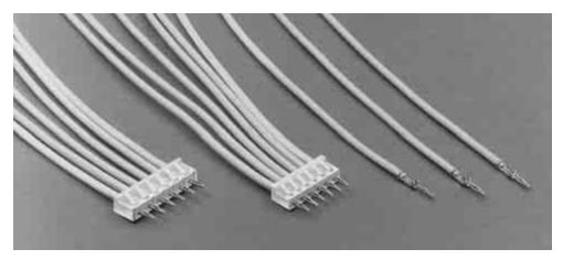
Low Profile Miniature AMP-IN Connectors provide an easy means of gang inserting leads into printed circuit boards. The design of the crimp snap-in contact aids in locating the pc board hole and inserting the contact into that hole.
