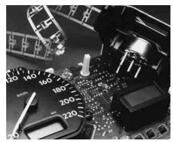
**Printed Circuit Board PCB Pin Receptacles**
