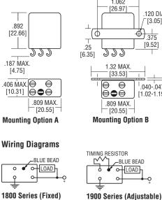
Note: The blank pin on 1800 series types is active and must not be connected
