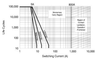
\*Based on extrapolated data. Since each application is unique, user is encouraged to verify rating in actual application. The load terminals should always be connected as follows: Common Contact (A2) positive; Other Contact negative.
