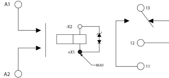
**NOTE:** Polarity must be observed with DC coil supply. Relay is polarized with a permanent magnet and will not operate or be damaged by reverse polarity.
