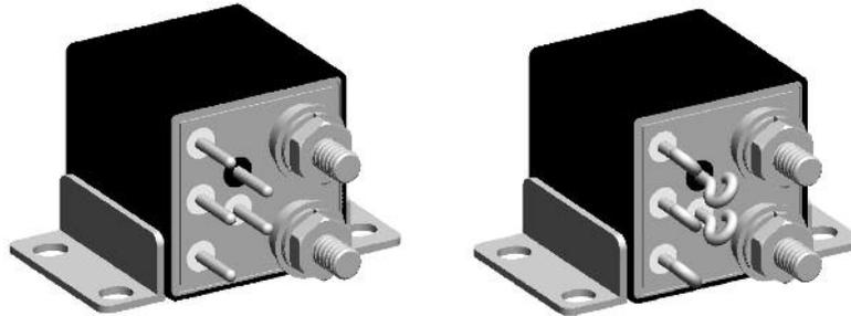
The FCAC-150 series relay is a polarized, single-side stable design, where the flux from a permanent magnet provides the armature holding force in the deactivated state, and its flux path is switched and combined
