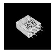
This relay has "memory" in that the contact positions do not change when coil power is removed. Switching is accomplished by applying power to the applicable coil (dual coil) or with the applicable polarity (single coil). The low switching power requirements are further enhanced by its ability to operate from capacitor discharge or other pulses or through its own contacts for batteries or similarly limited supplies.
