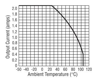
Figure 8 - Maximum Surge Current Without Tripping
