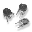
This tiny 6mm square cermet trimmer is offered with alternative adjustment covers for screwdriver and automatic setting and can be supplied in bulk or taped in ammo pack. The 416 trimmer can be adjusted from the top or side and is an inexpensive solution to high reliability potentiometer requirements. This series is used to replace some of the larger, expensive, sealed types in high volume circuits.
