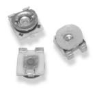
The 3135 miniature chip trimmer incorporates the latest technology developments and has been rigorously tested to the highest standards. It has been developed specifically for new generation handheld equipment, where the design specification demands precise setting and exceptional reliability. This tiny trimmer is supplied packaged for auto assembly in 8mm plastic blister tape on 180mm reels of 2000 units.
