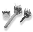
Tyco Electronics Components will customise these neat 16mm diameter control potentiometers to suit your requirements. They comprise a printed carbon resistance element with 0.25 W current handling and are available with various bush, termination and spindle styles
