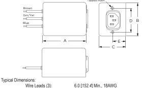
Line Inlet (1): Q8 Tapped Inserts (2): Q8M Tapped Inserts (2): 6.0 [152.4] Min., 18AWG IEC 60320-1 C14 6-32 x 1/4 M3 x .5
