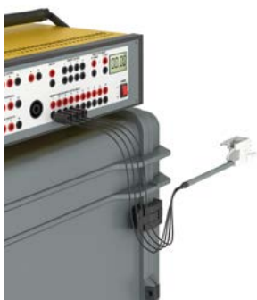
2.2 Connect the ESSAILEC® test plug leads to the test set.
