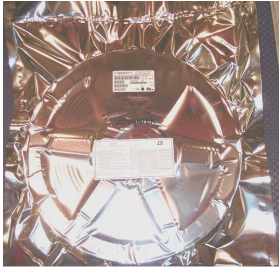
Fig. 2: Dry packed relay reel
