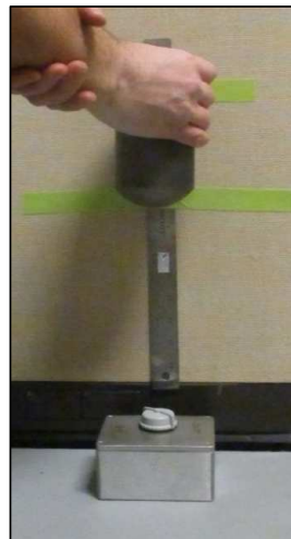
Figure 9 – Typical Impact Test Setup
