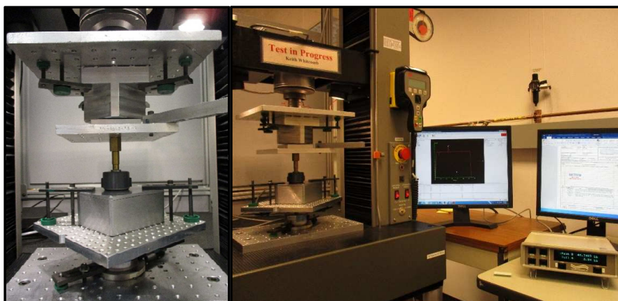
Figure 11 – Typical Receptacle Mounting Torque Test Setup
