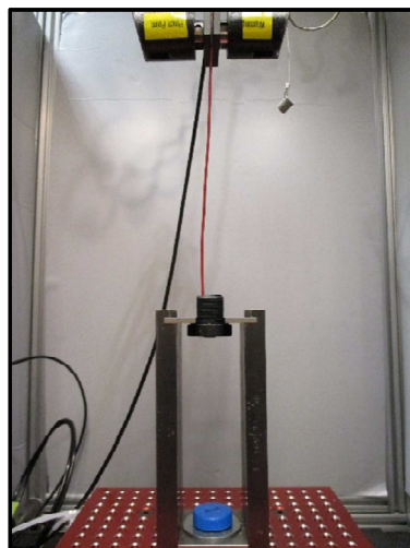
Figure 6 – Wire Retention Force Setup
