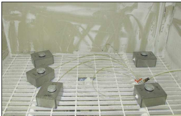
Figure 14 – Typical IP6X Test Setup
