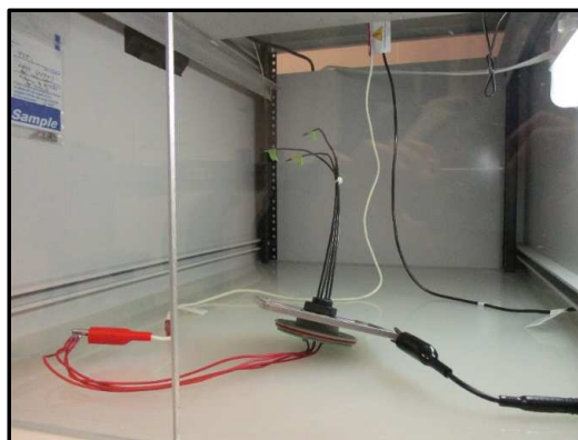
Figure 16 – Typical Withstanding Voltage – External Setup
