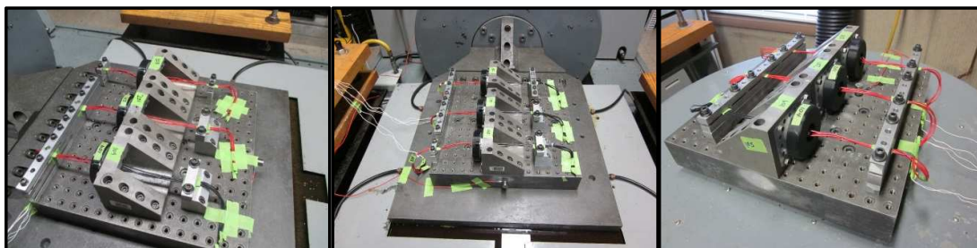
Figure 4 – Vibration Test Setup – X, Y and Z Axis
