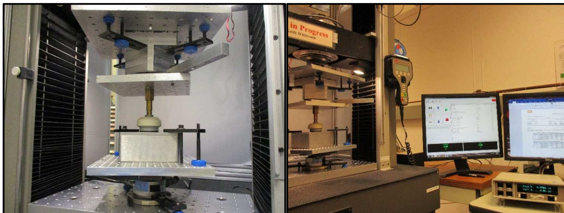
Figure 10 – Typical Mating and Un-Mating Torque Force Setup
