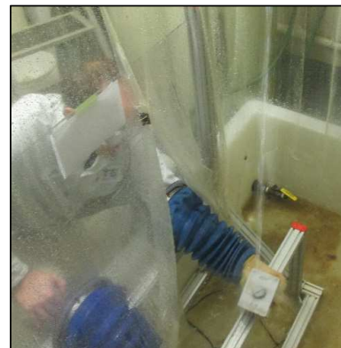
Figure 15 – Typical Ingress Protection IPX5 and IPX6 Test Setup
