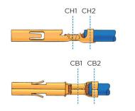
CH2: Insulation crimp height CH1: Conductor crimp height
