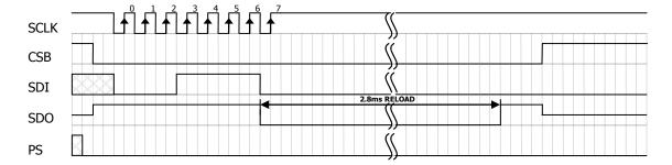
Figure 5: Reset command sequence SPI mode 3
