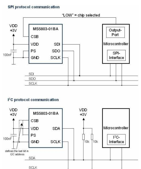
Figure 16: Typical application circuit with SPI /  $I^2C$  protocol communication
