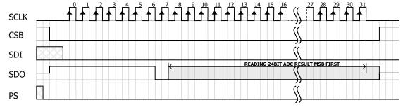
Figure 7: ADC Read sequence
