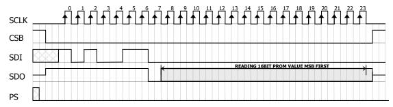
Figure 8: PROM Read sequence, address = 011 (Coefficient 3).
