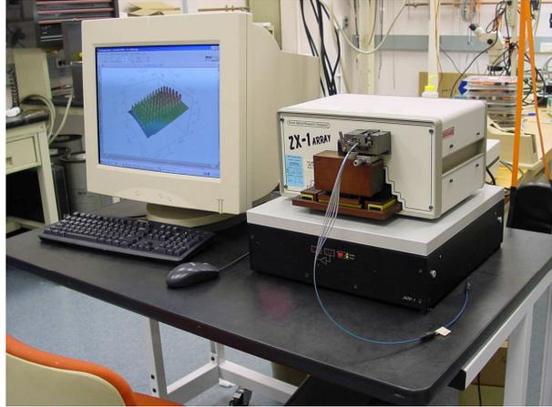
**Figure 6 – Equipment to measure end face geometry**
