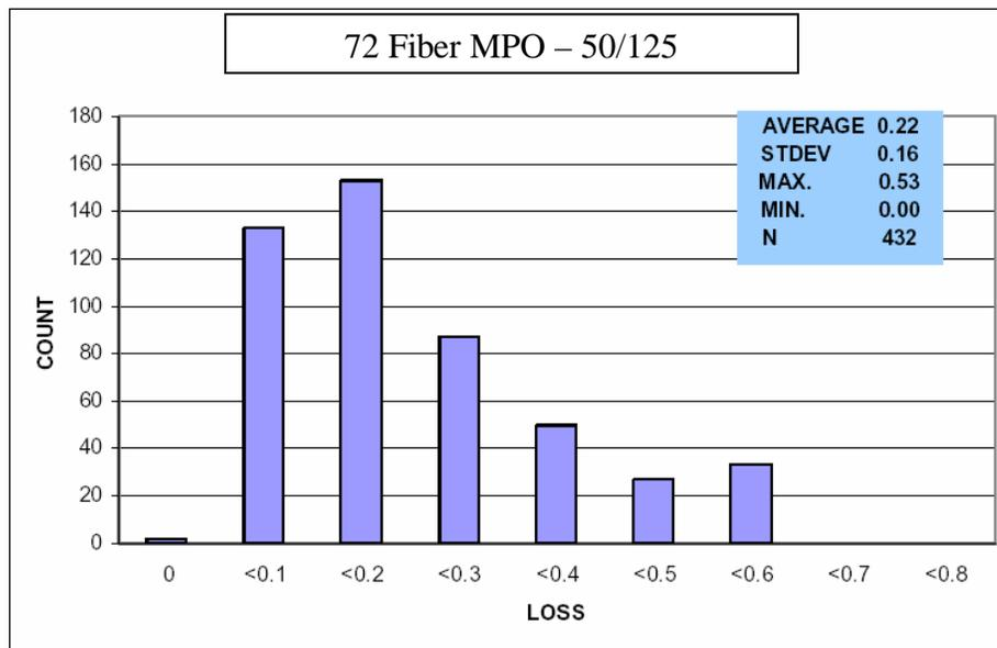
Figure 7 – 72 Fiber MPO Insertion Loss
