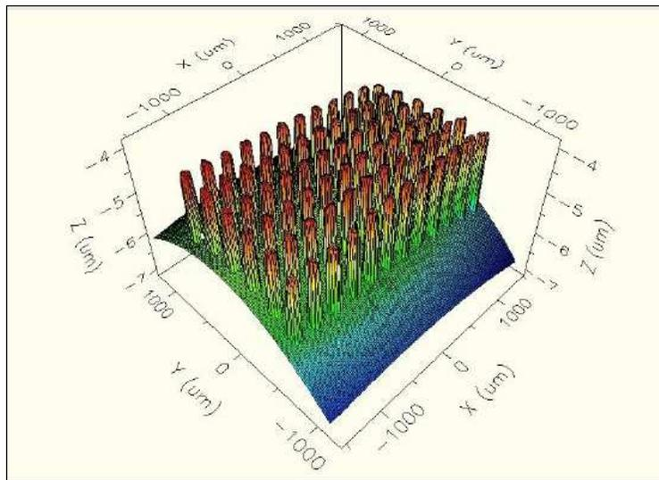
**Figure 5 – End face scan of 72 fiber MT ferrule**
