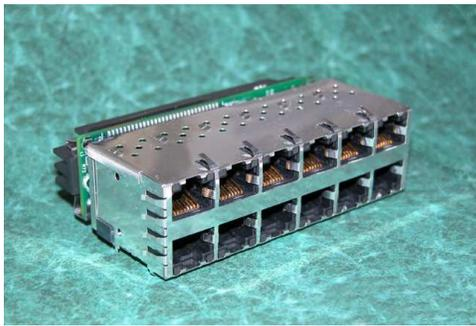
The first decision was to eliminate the existing soldered footprint and switch to a press-fit product. This eliminates costly wave soldering, and provides an easier migration to the European RoHS requirements for July 2006. The second was to provide the press-fit connector with a footprint that allows for easy migration between a magnetics only system, a PoE Enabled System (PoE devices separated from RJ45), and a PoE
