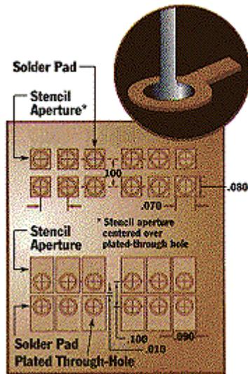
*The preferred solder joints show consistent, voidless coverage. Stencil apertures can be centered or offset over the hole.*
