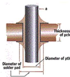
*The fillet volume must only be calculated once, since top and bottom fillets are assumed to be equal.*
