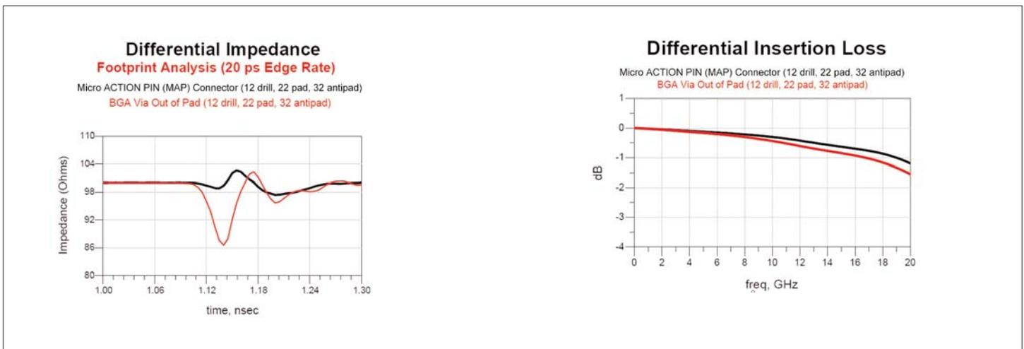
**Figure 5. Electrical performance comparison between MAP and BGA connectors**
