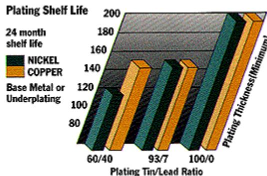
Eventually an intermetallic grows to the surface of the plating, where it oxidizes. An oxidized intermetallic layer will not solder.
