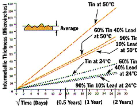
*Intermetallic growth, a leading cause of solderability failures, depends both on the composition of the tin plating and on storage temperatures.*
