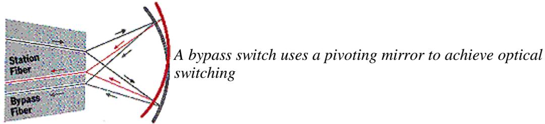
This CSR approach is highly stable, since the mirror can be pivoted to one of two highly stable positions. The fibers themselves, precisely placed during manufacture and coated with an antireflective coating to reduce back reflections, do not have to be moved.
