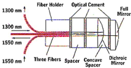
*A WDM uses two mirrors to direct two different wavelengths.*
