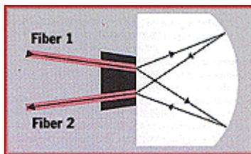
*CSR optics provides the 1:1 imaging needed for low-cost fiber-optic couplers.*
