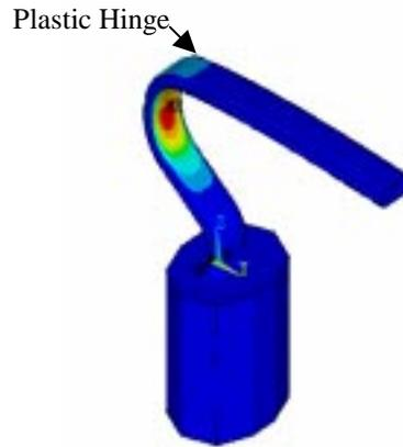
Figure 7: Contour plot of plastic strain
