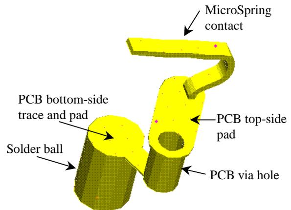
Figure 11 MicroSpring Contact Application
