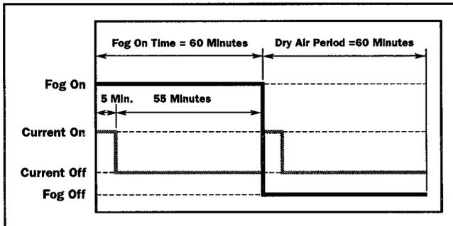
Figure 6. Current and salt fog cycles during harsh-environment testing.
