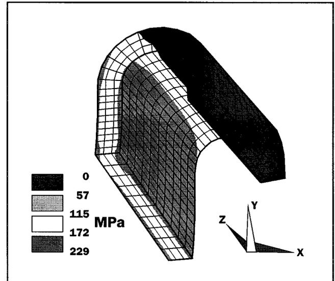
Figure 11. Computed von Mises stress distribution in the internal C-body surface.
