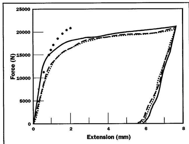
Figure 9. Typical force-displacement curves measured on unassembled C-bodies. Dots represent data calculated by FEA simulation.
