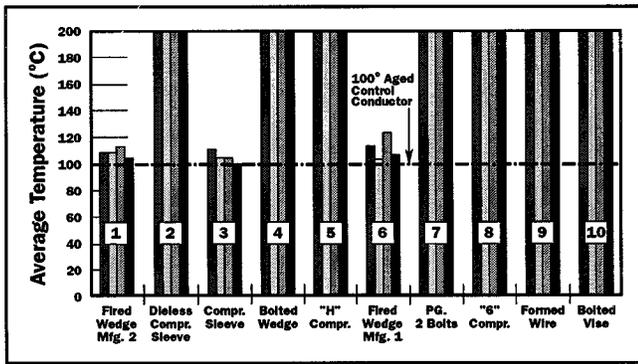
**Figure 4.** Connector temperature reached after a maximum of 129 current cycles, using *as-received/uncleaned service-aged* 397.5 kcmil AAC conductor.
