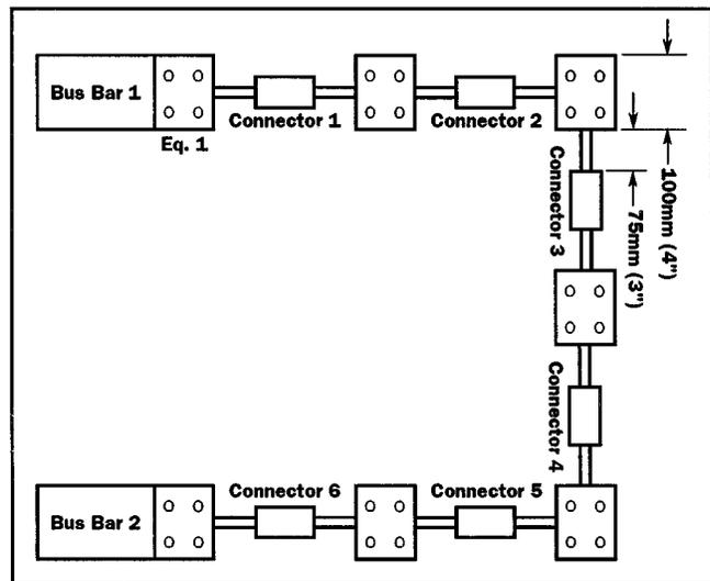
**Figure 5.** Block diagram of test loop in harsh-environment chamber.
