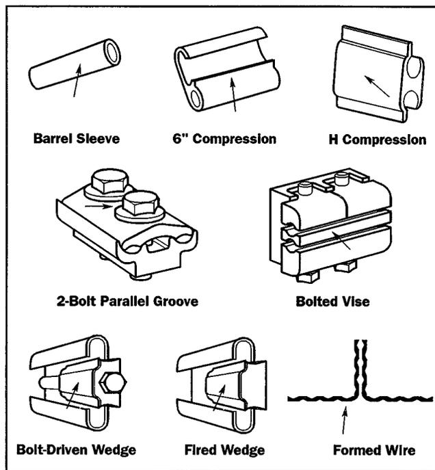
**Figure 1.** Schematics of tap-connectors evaluated in the present investigation.
