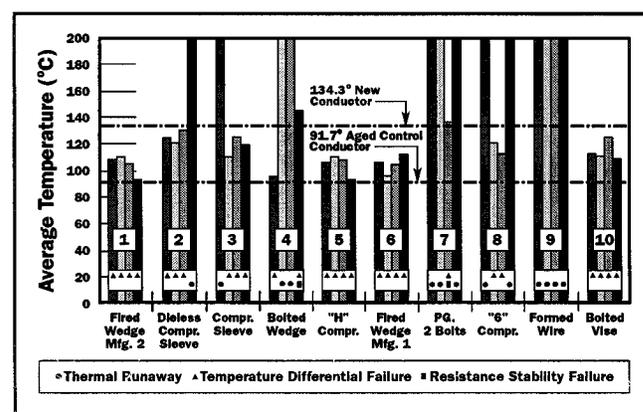
**Figure 3.** Connector temperature reached after a maximum of 129 current cycles, using *cleaned, service-aged* 397.5 kcmil AAC conductor.
