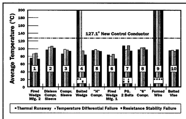
**Figure 2.** Connector temperature reached after a maximum of 500 current cycles, using *cleaned, new/unused* 397.5 kcmil AAC conductor.
