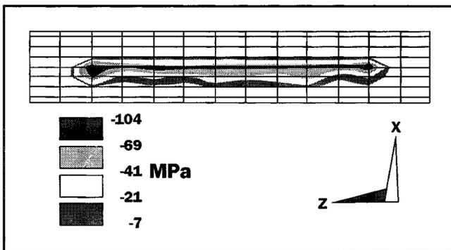
**Figure 14.** Computed contact stress distribution in the conductor surface mated to the wedge.
