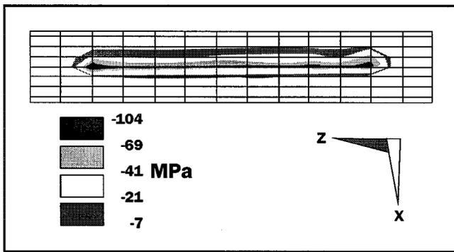
**Figure 13.** Computed contact stress distribution in the conductor surface mated to the C-member.
