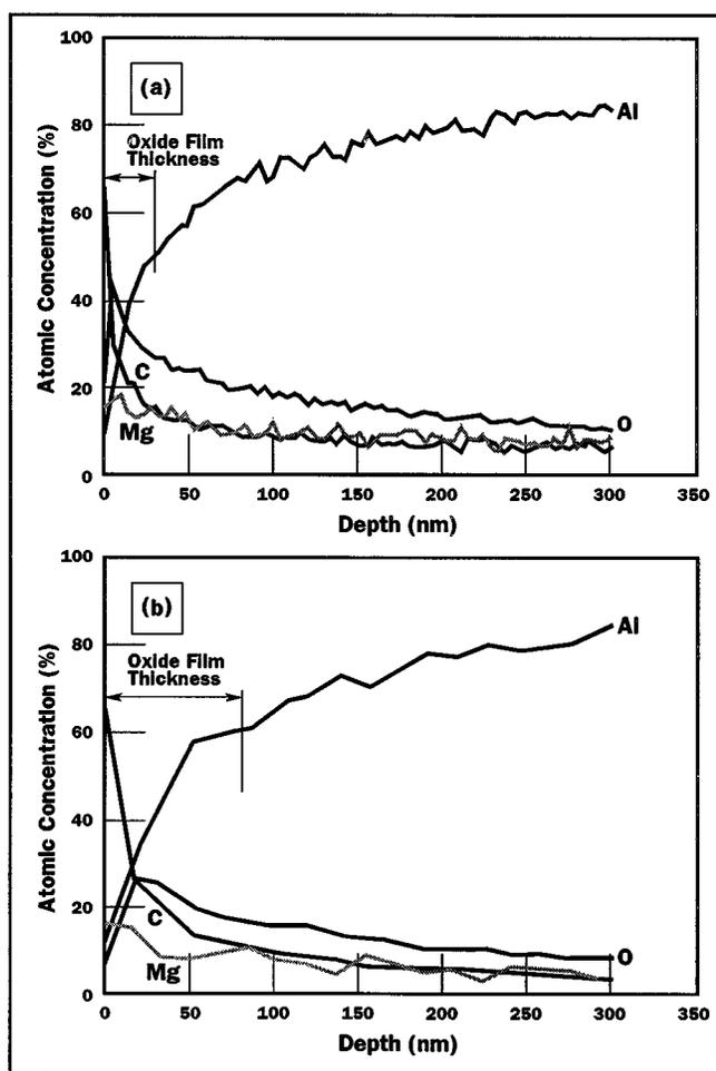
**Figure 16.** Auger electron spectroscopy depth profiles of (a) an abraded area on the wedge surface, (b) an unabraded area on the wedge surface. For definition of the terms abraded and unabraded used in this context see text.
