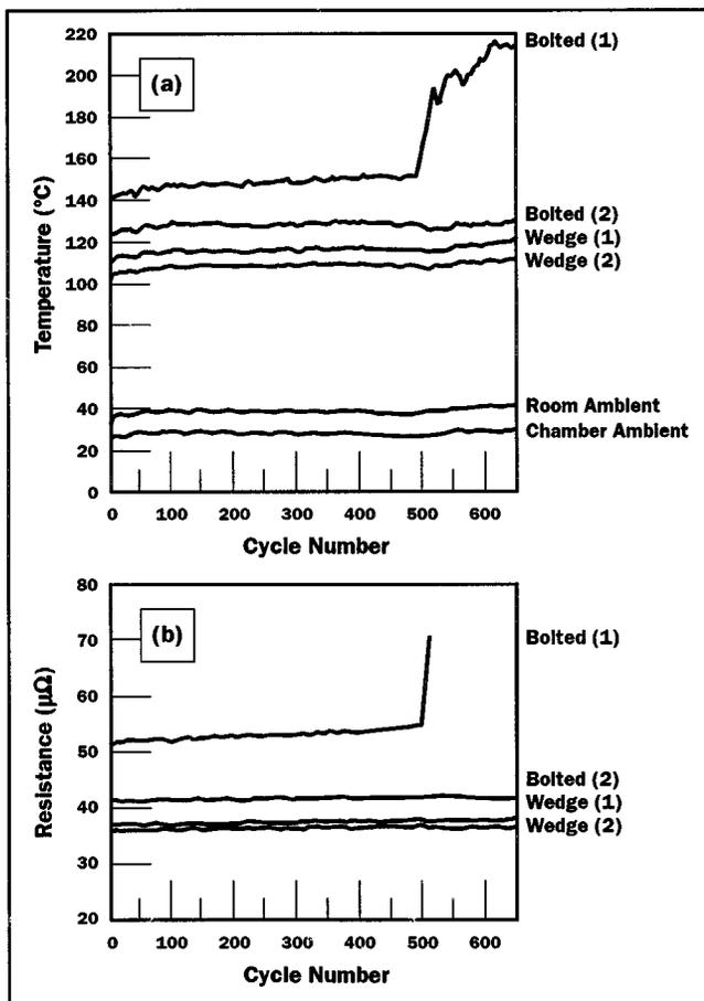
Figure 7. Typical results of harsh-environment testing. (a) peak connector temperature generated during current cycling. (b) corresponding electrical resistance variations.
