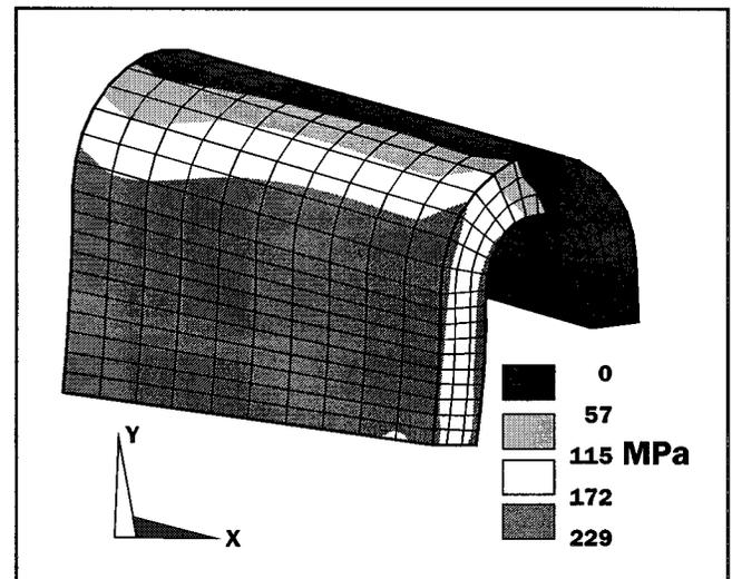
Figure 12. Computed von Mises stress distribution in the external C-body surface.
