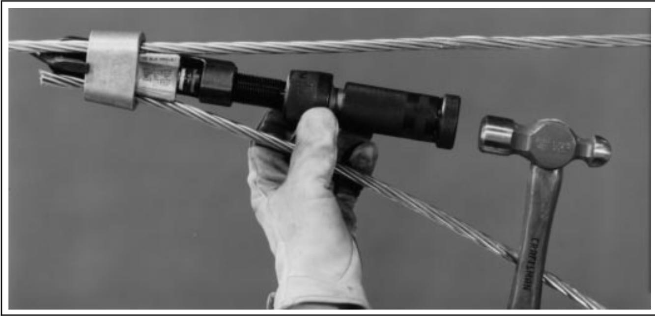
Figure 8. Wedge-connector installation with a cartridge-actuated tool.
