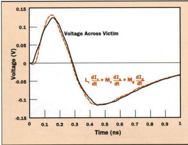
**Figure 11.** Comparison between the victim pin voltage drop and the sum of the inductive contributions to this voltage. It is obvious that capacitive coupling to the victim pin is negligible.
