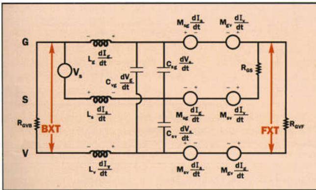
**Figure 5.** Single stage circuit model for three parallel pins allowing crosstalk and ground bounce. Measurement points for backward crosstalk (BXT) and forward crosstalk (FXT) voltages are shown.
