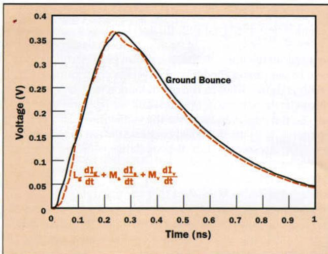
**Figure 12.** Comparison between the ground-bounce voltage and the sum of the inductive contributions to the ground pin voltage. It is apparent that the ground bounce can be attributed almost entirely to inductive effects in the ground conductor.
