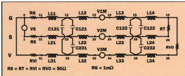
**Figure 6.** Two stage SPICE model for three parallel pins allowing for crosstalk and ground bounce. For simplicity, the coupling between the inductors is not shown.
