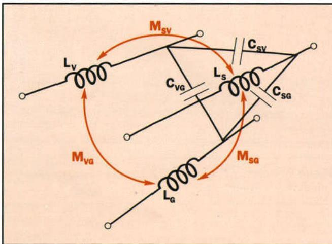
**Figure 3.** Practical equivalent circuit for differential section of two coupled transmission lines allowing crosstalk and ground bounce.
