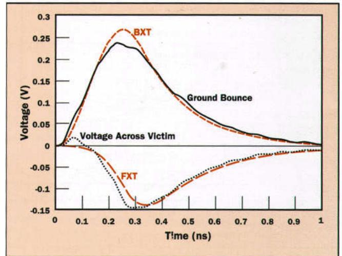
**Figure 13.** Ground bounce, backward crosstalk, forward crosstalk, and the voltage drop across the victim pin. Centerline spacings were reduced to 0.025 inch.
