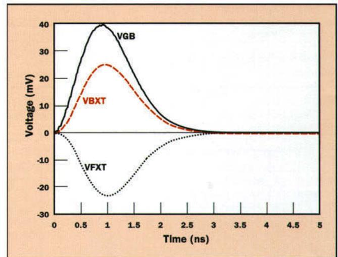
**Figure 7.** Ground bounce, backward crosstalk, and forward crosstalk for 1-ns risetime.
