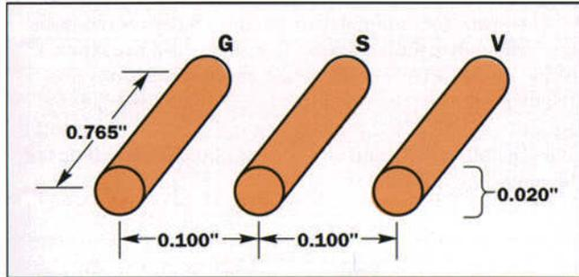
**Figure 4.** Three pin setup for analyzing crosstalk and ground bounce.
