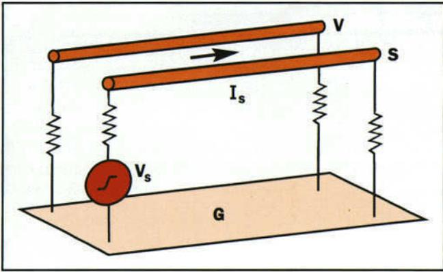
**Figure 1.** Two conductors sharing the same ground. A time-varying voltage  $V_s$  excites the signal conductor causing current  $I_s$ .
