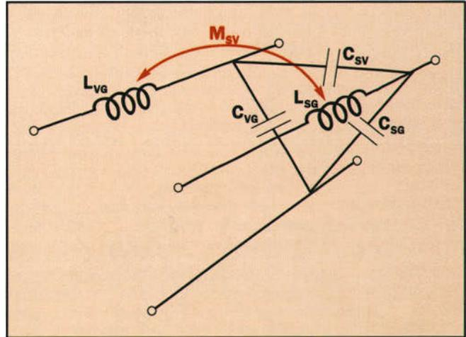
**Figure 2.** Differential section of two coupled transmission lines.
