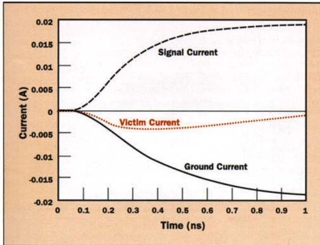
**Figure 8.** Currents generated across the three pins by the 200-Ps risetime step.
