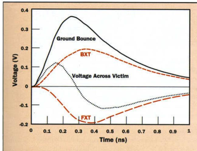
**Figure 9.** Ground bounce, backward crosstalk, forward crosstalk, and the voltage drop across the victim pin.
