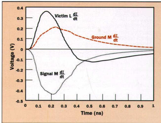
**Figure 10.** Voltages across the victim pin due to its self-inductance, mutual inductance with the signal pin, and mutual inductance with the ground pin.
