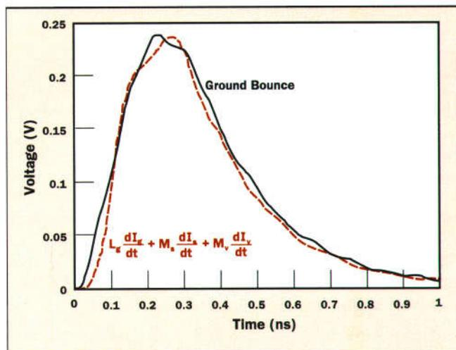
**Figure 16.** Comparison between the ground-bounce voltage and the sum of the inductive contributions to the ground pin voltage. Even with the reduced centerline spacing it is still apparent that the ground bounce can be attributed almost entirely to inductive effects.
