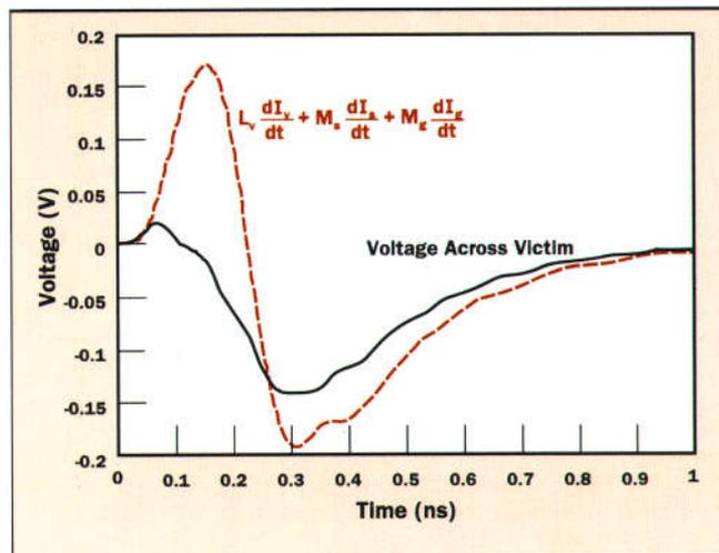
**Figure 15.** Comparison between the victim pin voltage drop and the sum of the inductive contributions to this voltage. Reducing the centerline spacing has caused a significant increase in capacitive coupling, which can no longer be ignored.
