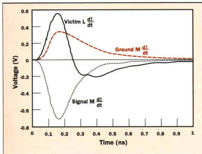
**Figure 14.** Voltages across the victim pin due to its self-inductance, mutual inductance with the signal pin, and mutual inductance with the ground pin. Centerline spacing is 0.025 inch.
