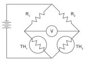
An example of bridge unbalance voltage vs. fluid flow velocity is shown in Figure 2. The bridge response is approximately linear at the lower flow rates. Measurement range is generally confined to flows in this linear portion.
