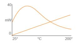
10. Note the point where the curves cross. This point is at 150°C and 20 milliwatts. Below this point (colder) there is more power available than required to attain that temperature and it will continue to rise. Above this point (hotter) not enough power is available and it will cool. Where the curves cross is the predicted stable point.
