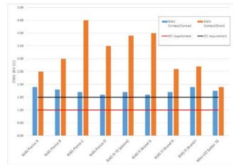
Fig. 5. Dielectric Withstanding Voltage - test until failure.
