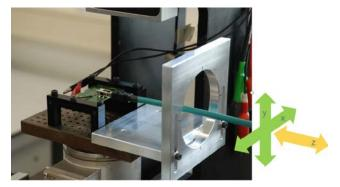
Fig. 7. Cable movement test set-up
