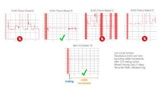
Fig. 8. LLCR during cable movement, test sequence exceeding IEC 60603-7-3.
