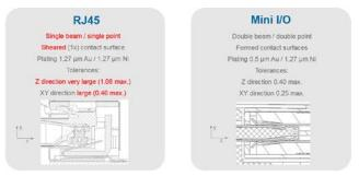
Fig. 2. Comparison of 2 Ethernet connector systems with cross sections of mating interface.
