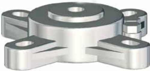
M5 Mounting base Pedestal Base with 4 slots to suit M12 bolts equally spaced on 127 - 140 PCD
