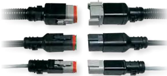
The DEUTSCH DT and DTM Series backshells are designed to snap onto and mate with all standard (basic plug and receptacles without modifications that affect the rear of the connector) DT and DTM Series connectors. The rigid, durable backshells offer a high level of protection and allow convoluted tubing to nest within the rear of the backshell. Straight (180°) and right angle (90°) versions and backshells with strain relief for jacketed cable are also available.
