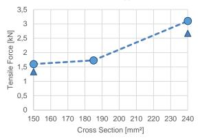
With bigger cross section comes a larger area where the copper plate can dig in the conductor material. With the bigger conductive and connecting area, both electrical and mechanical properties are better.
