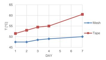
Here the temperature rise of the First Aid connector with tape becomes more evident. With the same test setup as current and ambient temperature, the maximum temperature of the tape design is 10 °C higher than the electrically optimized coppermesh-design.
