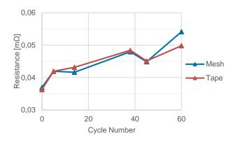
Electrical properties do not limit the performance of the First Aid connector. During the whole heat cycle, the DC-Resistance indicates an ageing process which is underlined by the steeper increase of the temperature. After 30 cycles, the First Aid connector according to tape design hits the limit of 65°C. The current has to be reduced then to 50% of load current.
