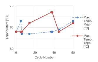
Now, it is evident that the tape ages faster than the solid copper mesh. During heating up, the tape becomes soft. As the insulation sleeve also loses interface pressure with rising temperature, the recovery force on the connection is lower. During this phase, the resistance is higher resulting in more heat losses. Consequently, the temperature in the connector is rising faster.
