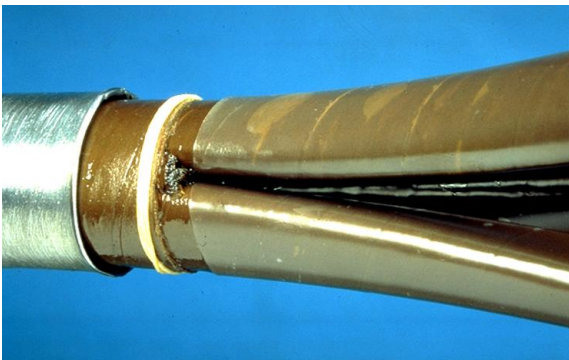
Figure 4. Oil barrier tube used in a 3-core paper cable joint
