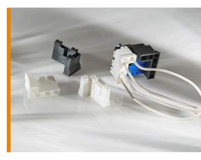
TE Connectivity (TE) introduces three and four position housings for use with Positive Lock Mark II receptacles or FASTON receptacles and M-style infinite switches. Infinite switches are rotary switches commonly used to control resistive heating elements and provide as many as seven .250 tabs for connections. Unlike some competitive housings, the new TE housings can accept one or two wires per receptacle.
