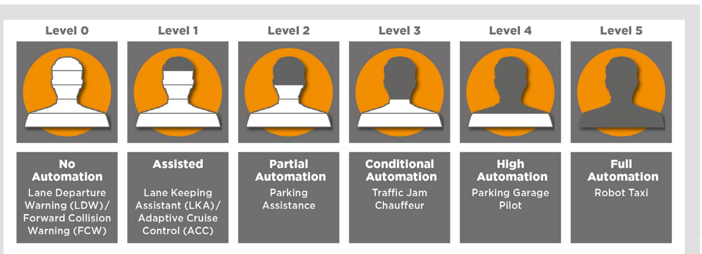
Figure 1: The levels of vehicle automation according to the Society of Automotive Engineers (SAE)
