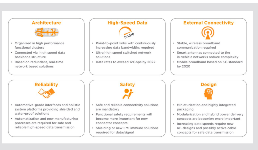
Figure 3: Six connectivity requirements of autonomous driving
