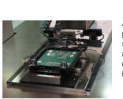
A key feature of the SEP press system is an automatic shuttle that positions the PCB and housing\connector stack up underneath the upper insertion tool.
