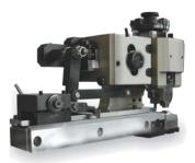
The FFC Applicator is designed for FFC and FPC terminations. It is normally delivered with a special Tyco Electronics crimp machine, but is also compatible with standard presses (press stroke 40 mm), if a wire feed is supplied.
