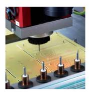
The GAS SAR-1000-B and SAR-1000-D depanelling systems for printed circuit boards and bare boards offers a largely automated process for depanelling by milling and/or sawing.
