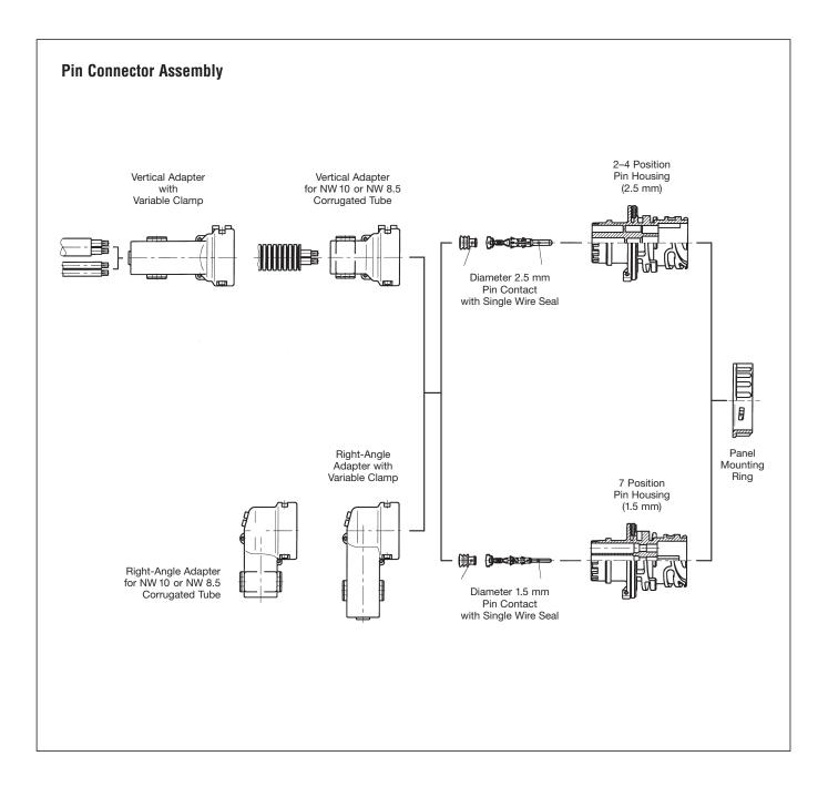
Sealed Diameter 1.5 mm/Diameter 2.5 mm Pin and Socket Housings
