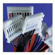
The IDC workstation produces electrical connections for harness assemblies specifically intended for the use within dashboard applications in the automotive industry. The proven insulation displacement technology ensures a high level of reliability. The software allows the production of different barrees
