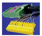
The development of this termination machine was necessary to be able to process high cavity-count female connectors in IDC technology. The new multicavity motor-control interface connectors are used in damp areas in cars and must be completely water-proof, hence the use of a family seal over the insulation displacement contacts.
