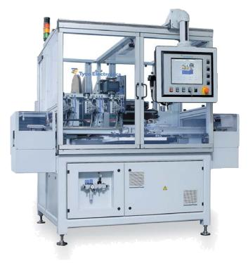
designed for easy use and provides the insertion force and a variety of production data to be collected at an open interface. With a maximum insertion rate of 4.5 cycles per second we provide a production capacity which is difficult to match in the market place. The programmable insertion of two 0.63 mm pins per cycle doubles the output.
