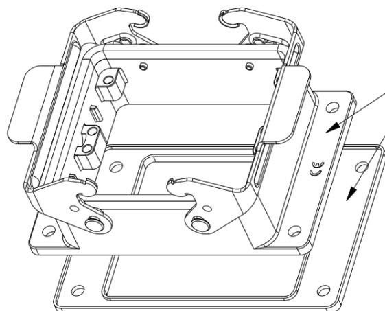
FLANGE SEALING SHOULD NOT BE STICKED TOGETHER WITH HOUSING. PUT TOGETHER SEPARATELY.
