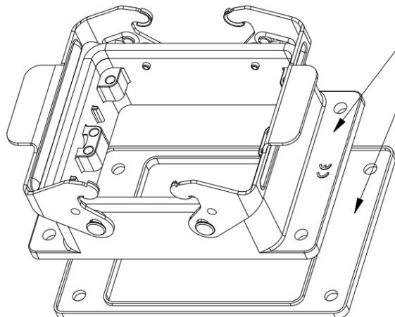
FLANGE SEALING SHOULD BE STICKED TOGETHER WITH HOUSING USING GLUE FULLY.
