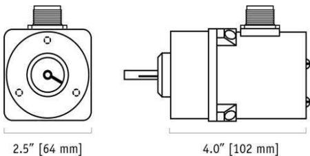
Celesco's model RT8101 provides a voltage feedback signal for rotational position. The sensing element of this device is a precision plastic-hybrid potentiometer which provides superb linearity and resolution.
