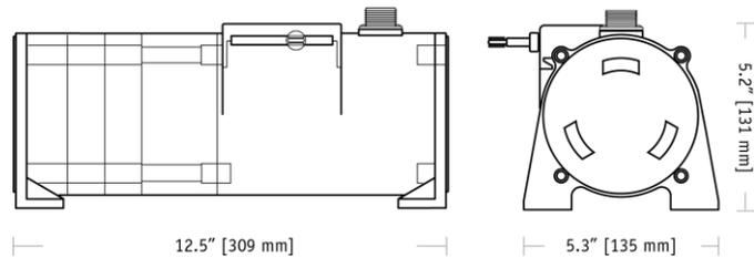
The PT9101 is a work-horse for demanding long-range applications requiring a linear position measurements in ranges up to 1700 inches. Available with either a 500, 1K, 5K, or 10K ohm potentiometer, the PT9101 operates with any basic panel meter or programmable controller.
