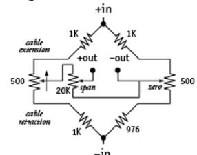
full scale output: adjustable from 0 to 30mV/V
