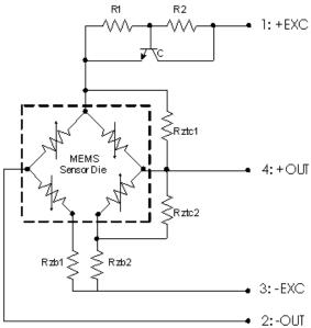
Note: Either Rzb1 or Rzb2 is installed, not both. If Rzb1 is installed then Rzb2 is shorted. Either Rtc1 or Rztc2 is installed, not both. If Rztc1 is installed then Rztc2 is left open.
