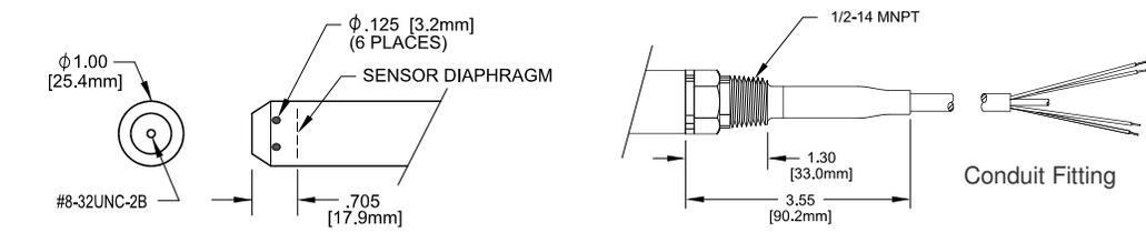
Molded Cable Seal Configuration for Polyurethane Cable
