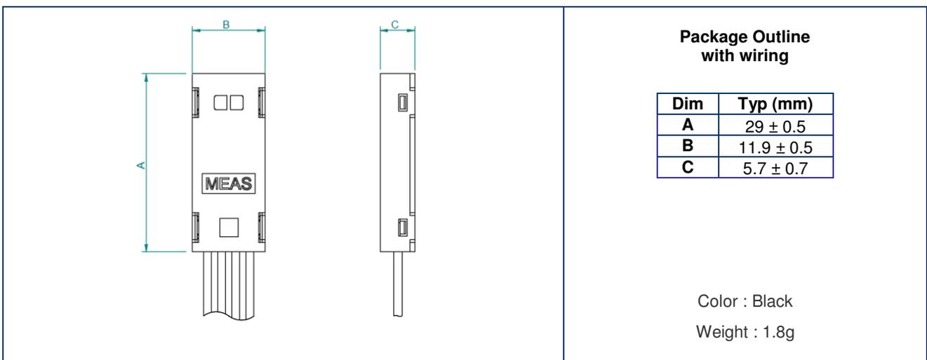
Double coated adhesive tape could be used on plastic housing area (ref: 3M – 5925F) to fix parts.
