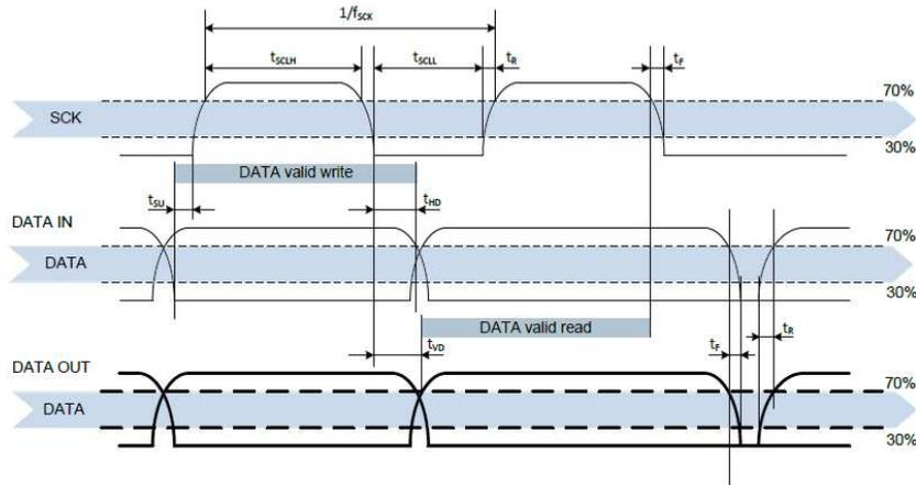
DATA directions are seen from the HTU3800 Series module. DATA line in bold is controlled by the module. DATA valid read time is triggered by falling edge of anterior toggle.
