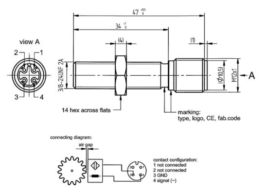
mates with straight plug M12x1, 4 pins
