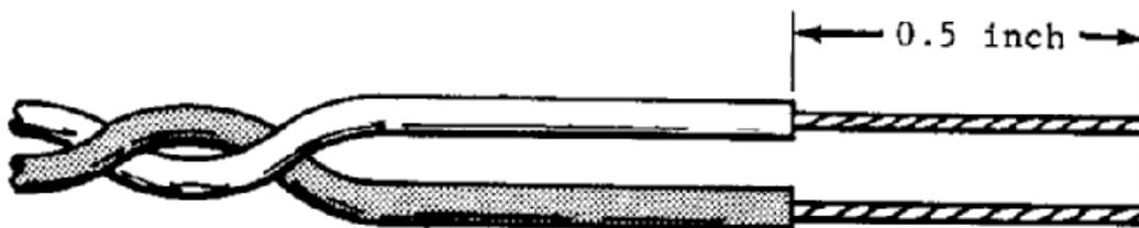
Figure 5-2. Wire Stripping Dimensions
