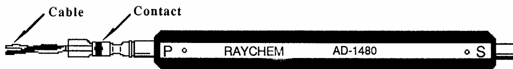
Figure 5-16. Contact/Cable Assembly Inserted into AD-1480 Holding Fixture (Outer Pin Contact Shown for Reference)
