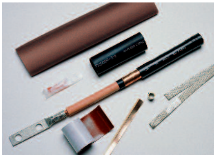
Cable with copper tape shield - grounding with roll spring and solder-blocked copper ground braid
