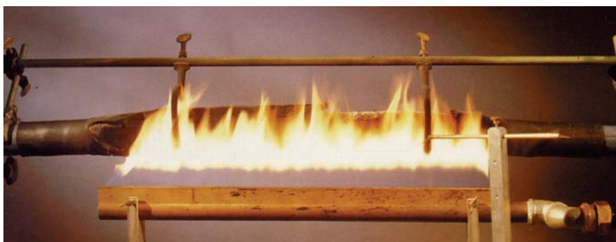
Photo 5: A fire-resistant Raychem joint maintaining its electrical integrity for more than 180 min. during a fire test according to IEC 60331.
