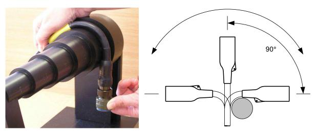
There should be no separation between the Moulded Part and the cable jacket at the adhesive bond line.
