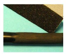
Figure 1 Degreased and abraded cable jacket
