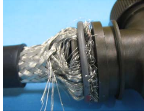
NOT ACCEPTABLE Shield weave not maintained
