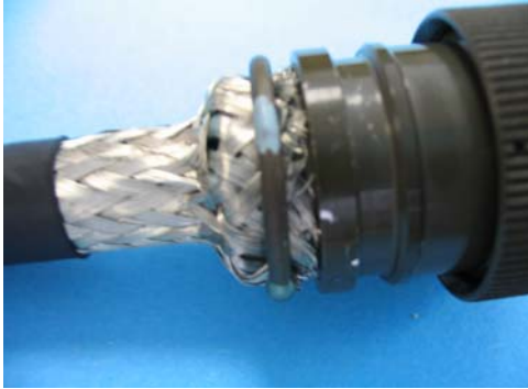
NOT ACCEPTABLE Ring not recovered, thermochromic paint unchanged in colour
