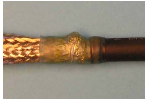
NOT ACCEPTABLE Shield spike penetrating Insulation
