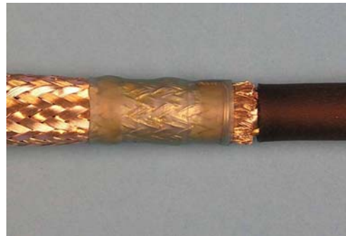
NOT ACCEPTABLE Solder sleeve incorrectly positioned
