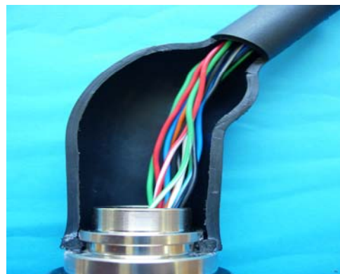
NOT ACCEPTABLE Insufficient strain relief
