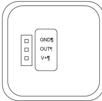
Figure 3: Pinning of the ED-18-XX-XXXX-X-X (bottom view)
