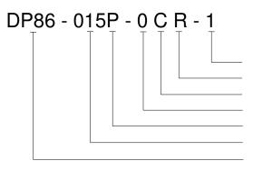
Cable (1 = No Cable on Pin Side, 2 = 1" Cable on Pin Side) Electrical (C = Ribbon Cable with Connector, R = Ribbon Cable) Type (C = Constant Current, Compensated) Fitting (Weldable, No Fitting) Unit (P = psi, B = Bar) Pressure Range Model
