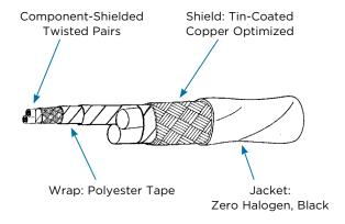
**Component:** Shielded Twisted Pairs **Shield:** Tin-Coated Copper, Optimized
