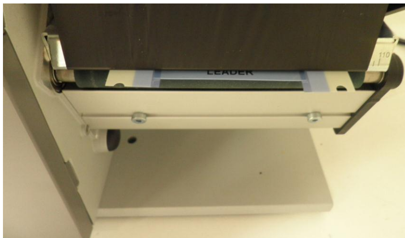
Figure 4, pull the markers back into the printer with the first marker showing
